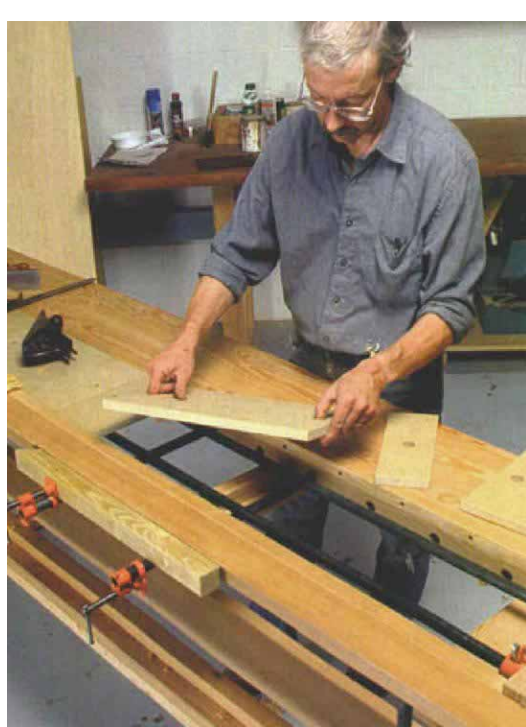
Lift-out MDF panels. The panels, cut in different lengths from MDF scraps, make a durable yet disposable center surface for the bench. The panels get removed when the tail-vice pipe clamps are in use.
