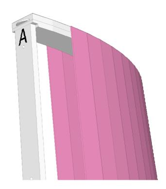
5. CAREFULLY SLIT THE PLASTIC ON EACH END OF EACH QUARTER SECTION. CAREFULLY PEEL BACK THE PLASTIC JUST ENOUGH TO EXPOSE THE HOLES THAT THE HARDWARE GOES THROUGH. YOU CAN REMOVE THE HANDWRITTEN LABELS IDENTIFYING LOCATION, TYPE OF SHADE AND DIMENSIONS. PLEASE MAKE SURE THAT NO RIBBON ON THE BOTTOM OF THE SHADE IS EXPOSED.
