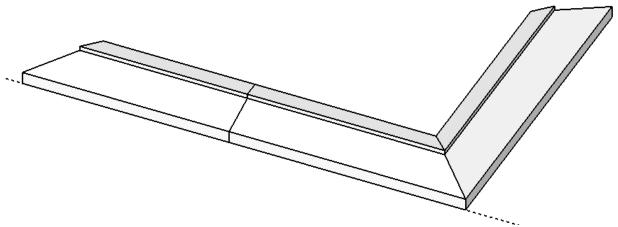
The lines joining the two portions of the long leg can be removed with the Eraser tool and perhaps the X-ray view. Draw a selection box around the resulting long leg and create a component.
