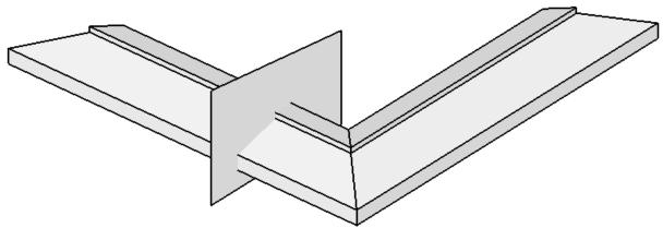
Separate the leg into individual lines/faces with Explode. Select the cutting plane and then Edit/Intersect/With Model to divide the leg into two pieces. The location (along the length of the leg) of the cutting plane is not critical. Delete the cutting plane. Draw a left to right selection box around the left portion of the leg. With the Move tool, select an outside corner of the miter and stretch it to the final long leg length of 12".
