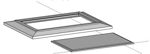
At the end, there should be four components in the model: profile, short leg, long leg, and panel. The legs should have mitered corners.
