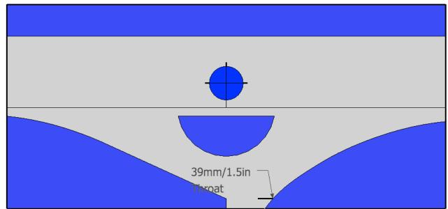
If things line up correctly the inside of edge A will rest against the bolt. If there is a tiny gap, loosen the nuts and clamp the bit in a vise with edge B facing upward. Gently adjust (bend) the cutting "wing" a in the direction of the bolt using a hammer or a large vise-grips. Retighten the nuts and check again.
