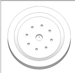
The new wheel with center hole and eight mounting holes.
