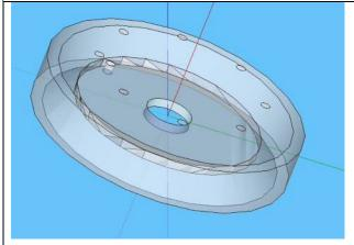
Here is an X-ray view of your wheel. You can see the internal faces. Not sure how you made this wheel. It is not a solid.
