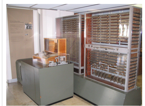
The first programmable computer, the Z3, included floating point arithmetic (replica on display at Deutsches Museum in Munich).
