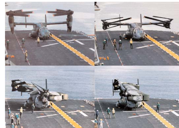
Blade Fold/Wing Stow Sequence
