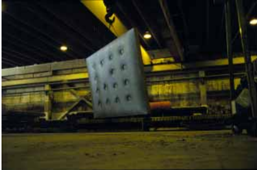
Figure 4. Another “direct-cast” concrete panel produced from the same lower frame and fabric formwork membrane as those illustrated in Figs. 1 and 2. In this case, however, intermediate supports were provided in a grid pattern. It will be noted that simple changes in intermediate support patterns will produce significantly different panel designs.
