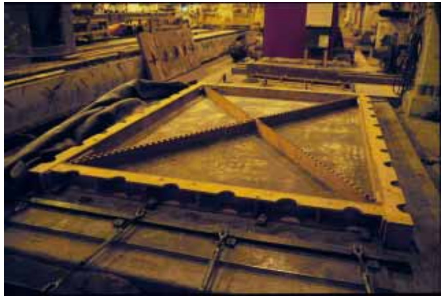
Figure 1. Lower frame with intermediate "X" support in place prior to placement of fabric formwork membrane.
