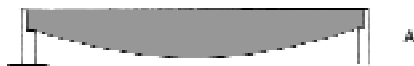
Figure 13a. Diagram of a vertical section through a direct-cast mold showing the funicular deflection of the formwork membrane caused by the weight of the wet concrete.
