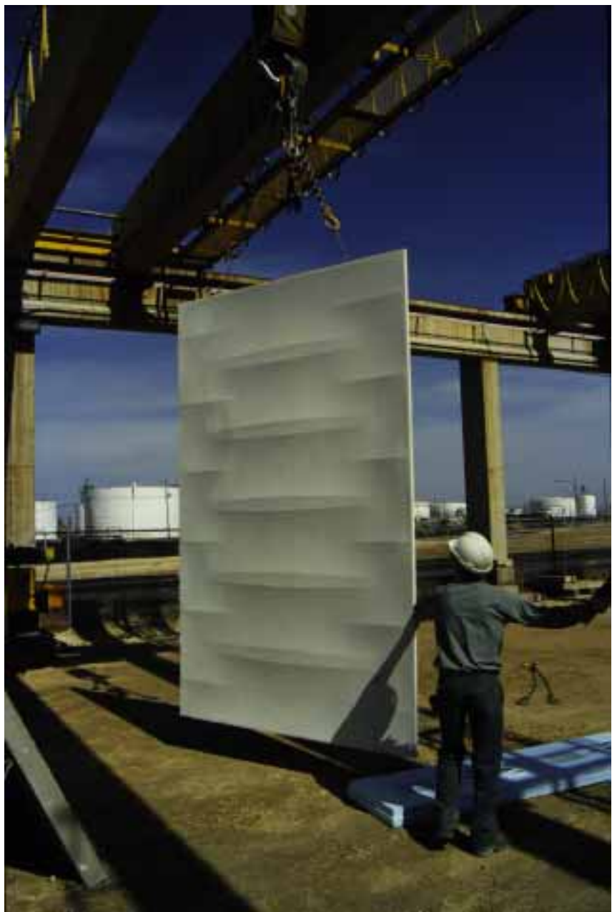
Figure 12. Lightweight GFRC shell panel produced from the Figure 11 “direct-cast” mold. This panel varies in thickness from 13 mm (0.5 in. ) to ( 38 mm (1.5 in.)).
