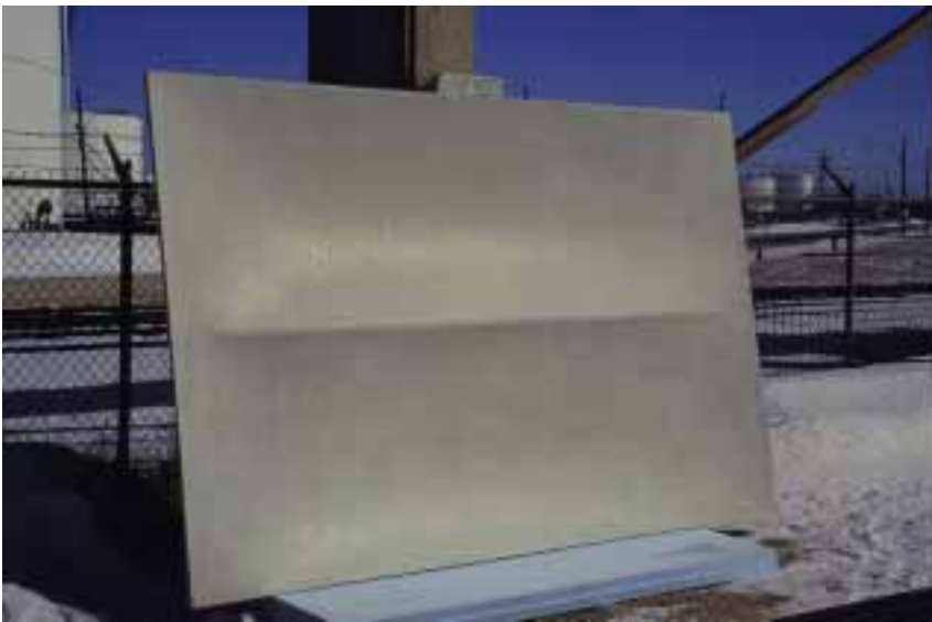
Figure 15. Lightweight GFRC shell panel cast from the Figure 14 mold.
