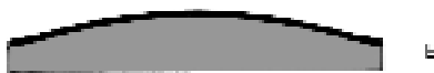
Figure 13b. Diagram showing the direct-cast mold inverted and used as a mold to cast a thin-shell panel (shown in black).
