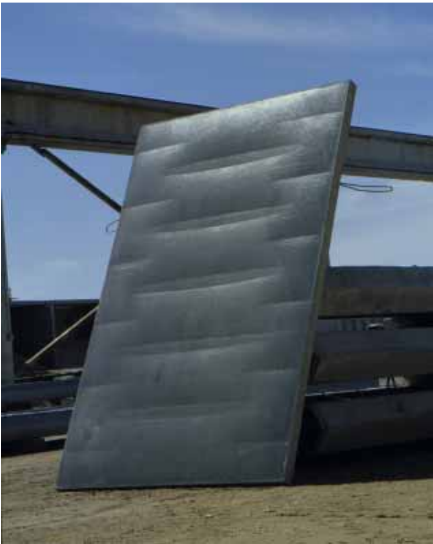
Figure 11. Fabric-cast mold for the Figure 12 GFRC shell panel. This mold was produced from the Figure 10 intermediate support design.
