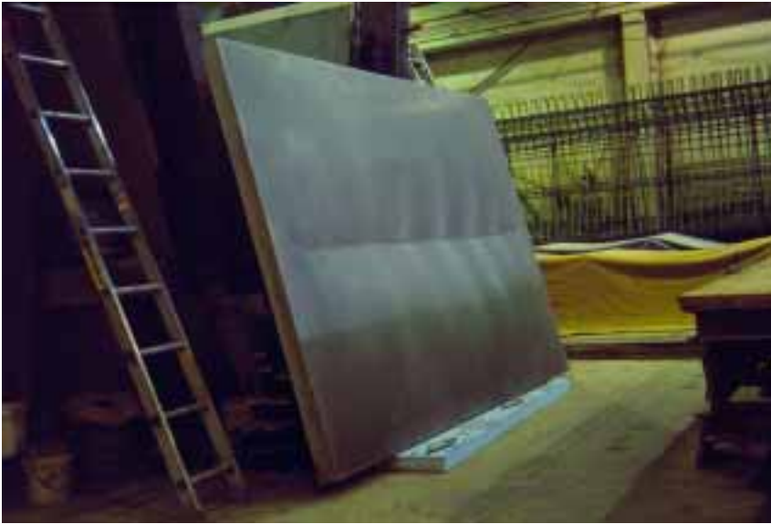
Figure 14. "Direct-cast" mold used to produce the Figure 15 GFRC shell panel.
