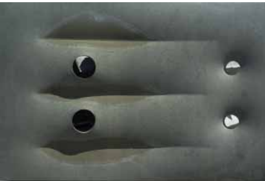
Figure 7. The “direct-cast” concrete panel formed from the formwork shown in Figure 6.
