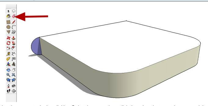
Using the eraser tool plus clicking Ctrl at the same time, click the edges between the arcs and the straight edges.
