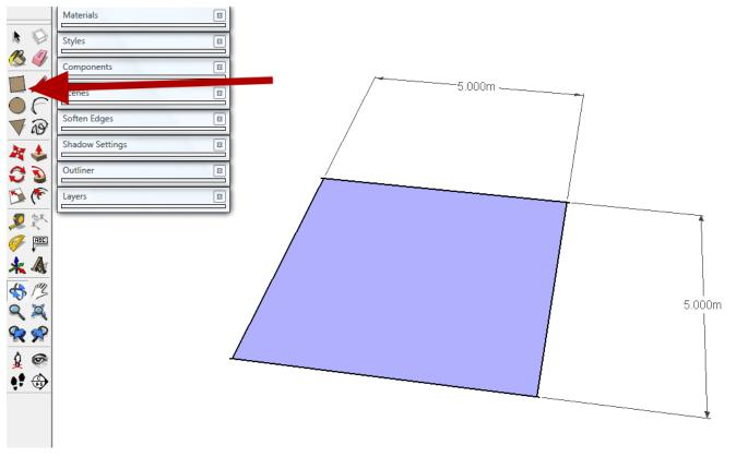
Use the tool the arrow points to. The square can be of any size, but mine is 5m x 5m, because big means you can add more detail.
