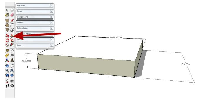
To push-pull, use the tool the arrow points to. You can push pull any distance, but make sure it's not a box.
