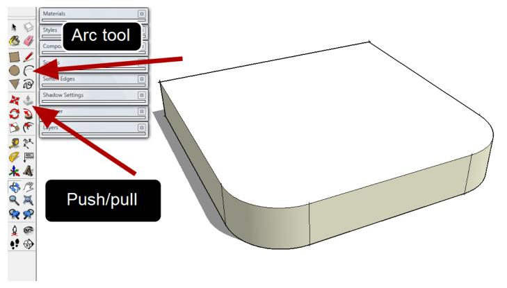
Use the arc tool to make two arcs. Then, copy the arc by using the move tool while pressing Ctrl at the same time. After that, push pull down the two arcs.
