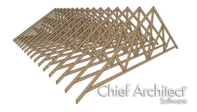
Drawing roof trusses in Chief Architect is as simple as drawing and replicating a line - as long as certain conditions are met. Roof trusses in the program are defined by the position of one or more roof planes above and one or more ceilings below, so both must be in place before a truss is drawn.
