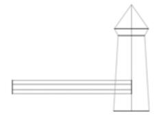
Switch to the front and right views to ensure the overlap is there. Now select both the tower and the extrude and select the Subtract Surface from the Model menu...
