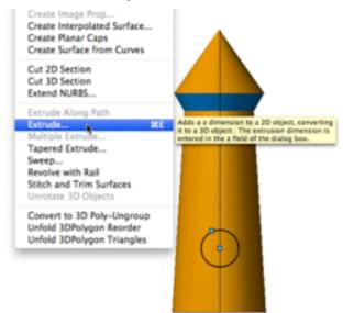
Extrude to something like 5000. Switch to Top/Plan view. This will turn off the rendering and switch to a wireframe view. Check to make sure that the extruded circle is overlapping the tower shape.
