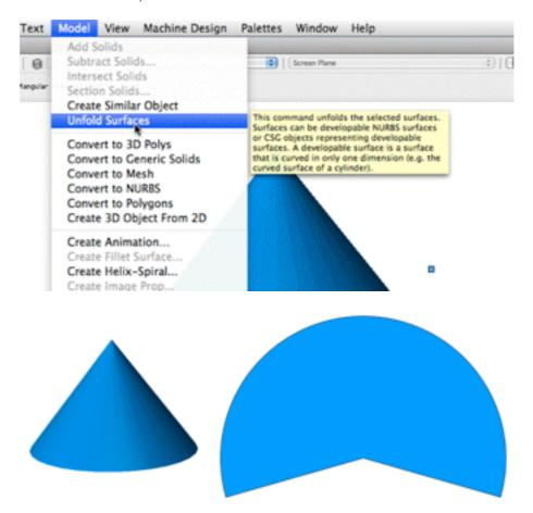
The result is that VW creates a flattened version of the NURBS surface. To use this in the real (fabric) world, you'd need to use something like Aeronaut's Add Seams plug-in to add the right seam allowances. Since this process removes the pattern colour, it's probably best left until last.
