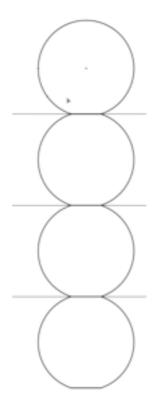
If you use the above technique without modification, you will end up with acceptable results, but when the tubes are unfolded, you will end up with several segments from each tube. When VW performs the flattening operation, you get one segment from the curved section of the tube and another segment from the gusset or flattened part of the tube.
