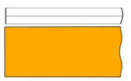
Notice the left end of the flattened extrude... it's exactly the shape you would expect to get when a coned object intersects a cylinder.
