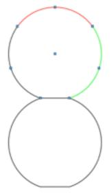
Delete the red and green segments. Click on the end of the remaining segment and drag the end around so it meets the flattened base line. Repeat the decompose on the lower shape so each side is one arc.
