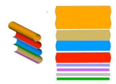
Add seam allowances to suit. Once the pieces have been correlated with the original colours on the extrude, they can be numbered, strike-up marks added if desired, and then they can be converted back to their proper colours for exporting and nesting.
