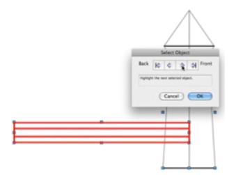
Click on the arrows until the extruded circle is highlighted. Then click on OK. The tower will be subtracted or clipped off the end of the extrude. The tower will probably disappear... that's why we duplicated it to begin with.
