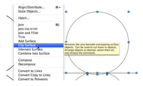
The result should look this: The lines can be deleted and the tubes extruded clipped and flattened as shown earlier.
