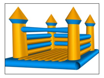
Most of the shapes used in this model are extrusions or sweeps. The towers are very simply made from a few sweeps. A sweep, sometimes also called "lathe" is used to make a surface by rotation. In VW, the centre of rotation is located with a locus. Before you perform anything in 3D, switch to the view you need for your model, in this case it's the Front view.
