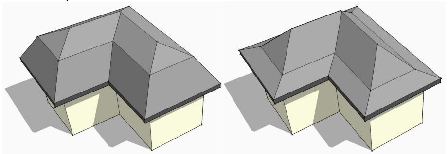
See the general guidance for Hipped Roof above... This tool gives a roof with two pitches, with a crank at a given height above the eaves. The dialog differs from the Hipped Roof Tool in that two angles are entered for the lower and upper roof pitches and you also enter a height above the eaves level for the crank in the two pitches...
