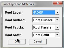
In a second dialog suggested layer/material names are shown with <default>s and pre-existing layers/materials listed. If the layer or material ('Roof xxx') that is picked does not exist then it will be made. You can pre-make or edit these later and they will be then used as you've set them.
