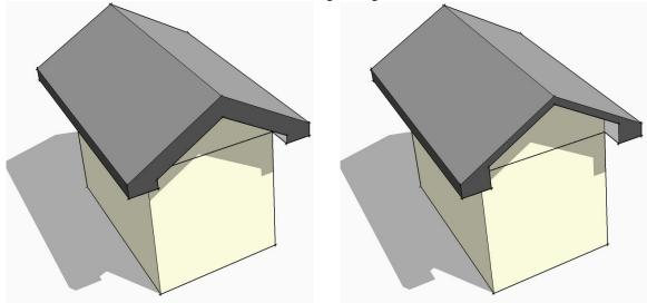
'Verge by Height, with Box-Eaves' - As 'Verge by Height' above, but also makes a boxed fascia using the fascia and soffit sizes along the bottom edge, its material [if any] will match the fascia.
