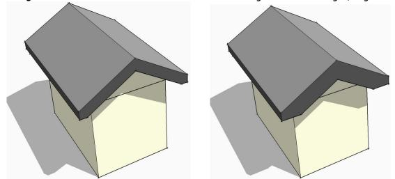
'Verge by Height' - this defaults to the eaves-fascia depth (or if this is 0 to 100mm/4") to make the verge (barge-board), you must enter a new value > 0 and < 'height of roof apex above fascia', its material [if any] will match the fascia.
