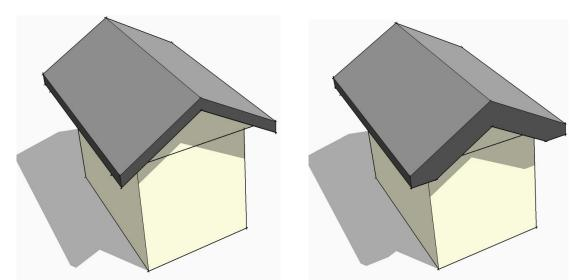
'Verge from Fascia' - this uses the eaves-fascia depth to make the verge (barge-board), its material [if any] will match the fascia.
