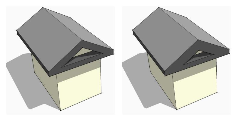
'Verge by Height, with Fascia' - As 'Verge by Height' above but also makes a fascia along the bottom edge, its material [if any] will match the fascia. 'Verge by Width, with Fascia' - As 'Verge by Width' above but also makes a fascia along the bottom edge, its material [if any] will match the fascia.
