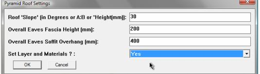
In this dialog enter the details: firstly the roof slope - as an angle in degrees
