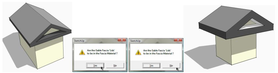
'Verge with Fascia [All Equal]' - As 'Verge by Width, with Fascia' above but also makes a fascia along the bottom edge with the same dimension (no dialog), its material [if any] will match the fascia.
