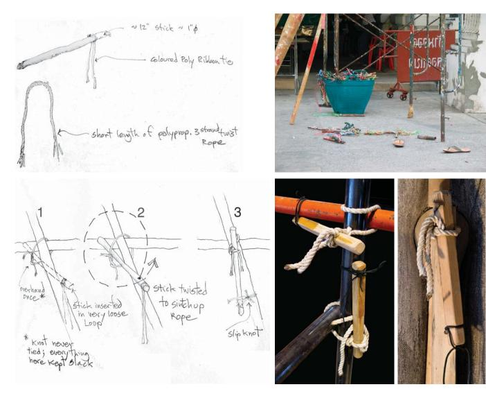
The connector parts are bundled together for storage and transport: one stick + one rope, bound together with the small tie that is attached to the stick.
