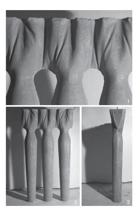
The C.I.P. screen wall is designed to form a series of small vertical columns joined by a horizontal beam that connects the tops of these columns and forms an open screen. The openings in the wall allow air and light to filter through the wall while reducing self-weight and consumption of raw materials.
