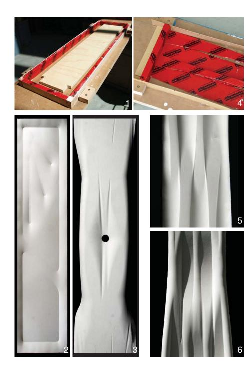
Strategies for reducing concrete in the central portion of a direct-cast panel include providing a slightly raised "table" inside the mold's edge frame (1). The deeper troughs created between the edges of this 'table' and the frame form the panel's edge beams. Further low-relief impressions (2), may be formed by placing objects on the 'table' or by changing the profile of the table's edges.
